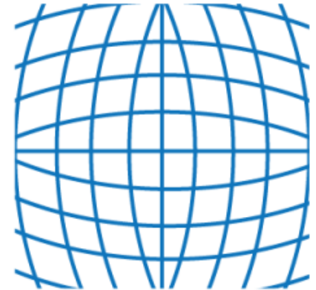
positive radial distortion "barrel"
