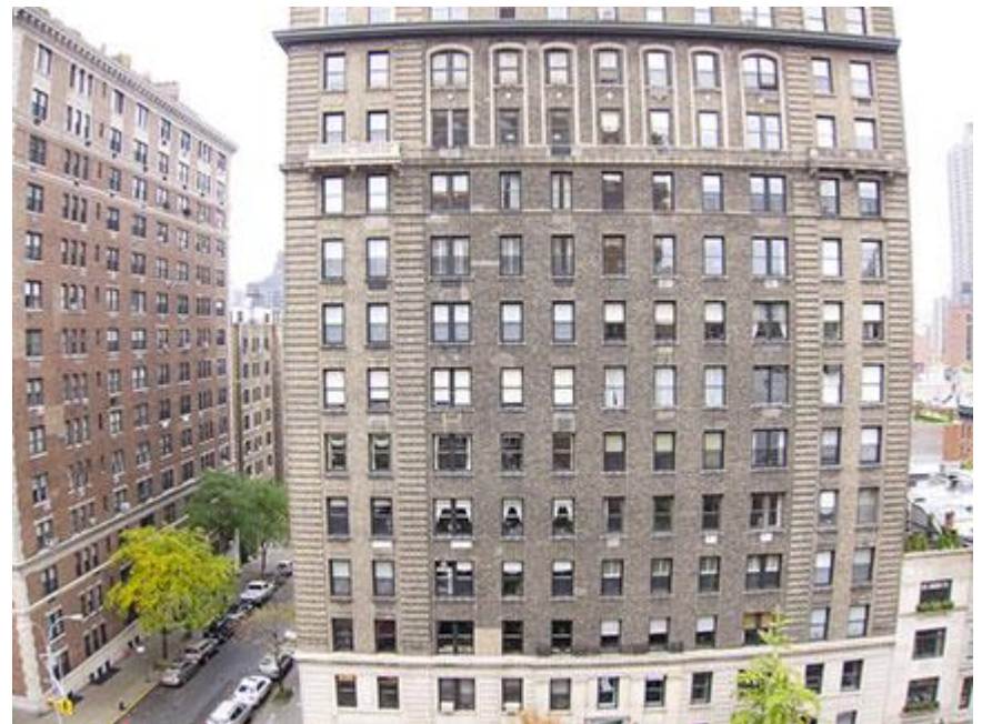
positive radial distortion "barrel"
